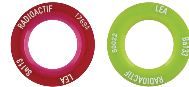
For A and E types, the distance between the active part and the height of the ring is 0.08 in.
